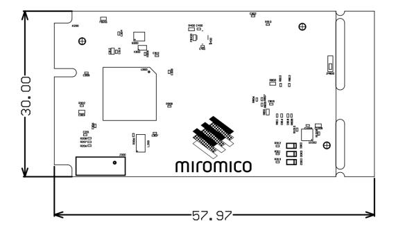
Figure 2: Top view, all values in mm
