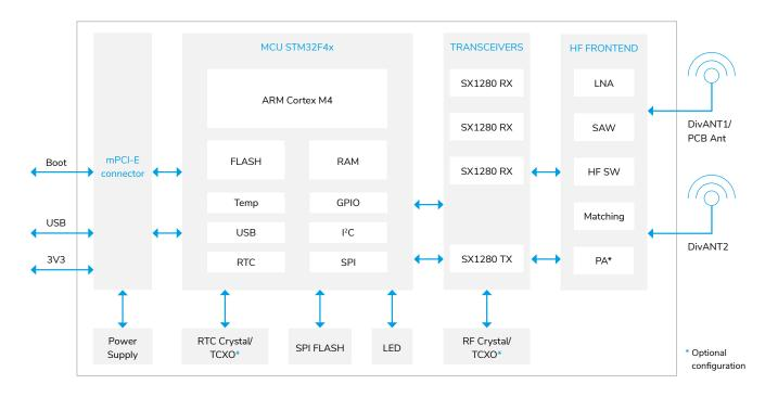
Figure 1: Block diagram miro EdgeCard
