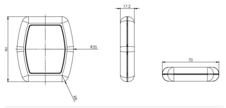
Figure 1: Mechanical Dimensions in mm
